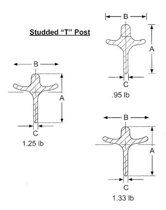
**Material:** Posts are produced from standard "T" rails weighing 91 lbs/yd or more according to ASTM A499 Grade 60; or ASTM A702 (1.33 lbs/ft only).
